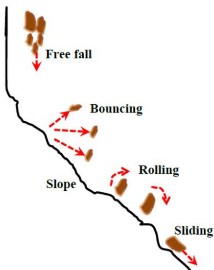
Fig. 1. Types of motion during a rock fall [1].
