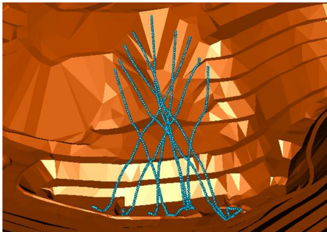
Fig. 3. Slope geometry affecting the fall body trajectory.
